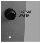
Safety thermostat with manual reset for the water temperature: if the temperature of the water tank exceeds the preset safety level of 85 °C immediately stops the operation of the thermostove and the display will show "ALAR-SIC-FAIL". To restart you need to reset manually.
