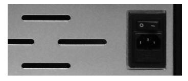
mean that the service fuse needs replacing. On the rear of the Thermostove there is a fuse holding compartment which is located underneath the supply socket. With a screwdriver open the cover of the fuse holding compartment, and re place the fuse if necessary (3,15 AT delayed type). Plug the unit back in and press the main switch.
