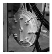
**Pressure switch:** monitors depression in the smoke duct. It is designed to shut down the pellet feed screw in the event of an obstructed flue or significant backpressure in the presence of wind. At the time of the pressure switch will show "ALAR-DEP-FAIL".
